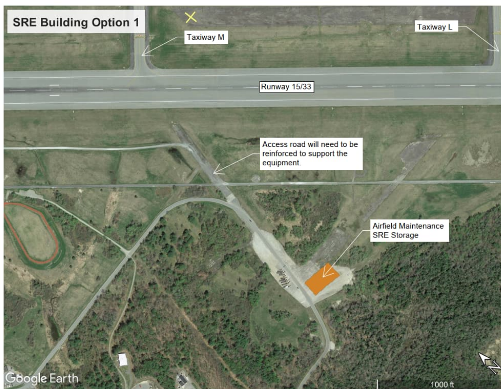
Figure 6-6. Maintenance / SRE Building - Option 1
