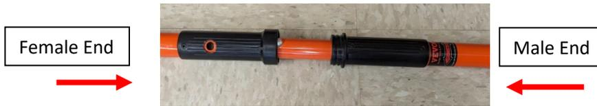
2. Once the two black plastic section are touching, engage the plastic threads and screw the two sections together
