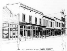
Figure 1. Inappropriate storefront alterations over the years—metal cladding, oversized signs and canopies—have detracted from the character of this historic district in Van Buren, Arkansas. A carefully considered rehabilitation plan for Main Street, including the removal of poorly designed signs, false fronts and the selection of an appropriate exterior paint color palette, serves to enhance the visual environment and preserves the district's sense of time and place. Photo above: Bob Dunn; Drawing: David Fets.
